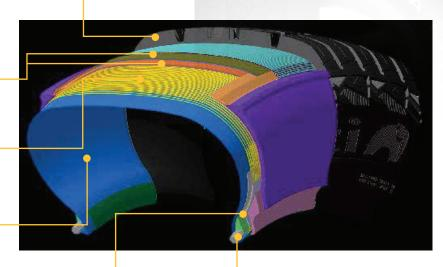
Bead wire Single wire winding technology to enhance the strength of the tyres bead and reduce the appearance of fatigue effects
